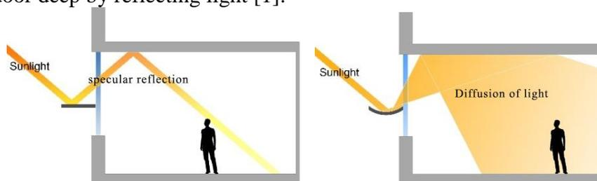
**Figure 1.** The principle of the shelf system of light & the principle of application light shelf system of curvature
