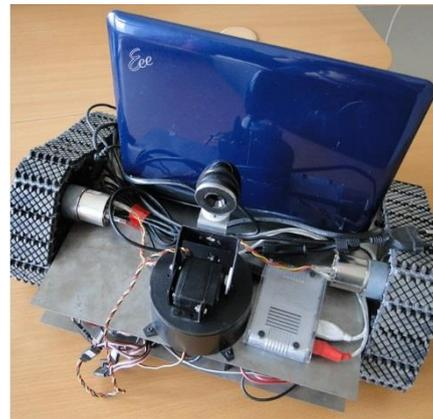
Figure 4: Mobile robot Kuzma II.3
