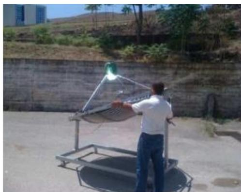
**Figure 2:** Picture of the concentrator with cylinder mounted as receiver
