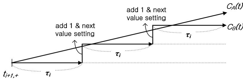
Fig. 1. Process of skew compensation
