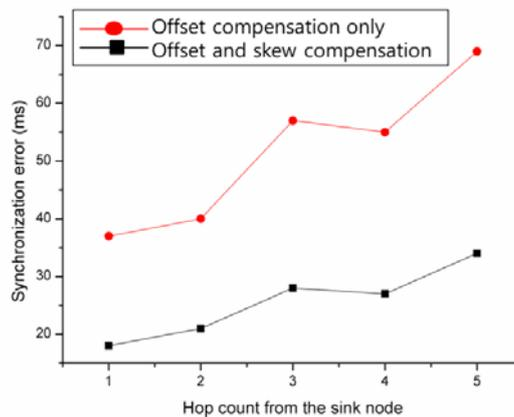
Fig. 2. Synchronization errors at each offset and skew compensation cases
