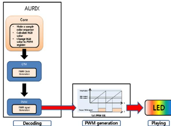
Fig. 2. Operation block diagram of dynamic LED system
