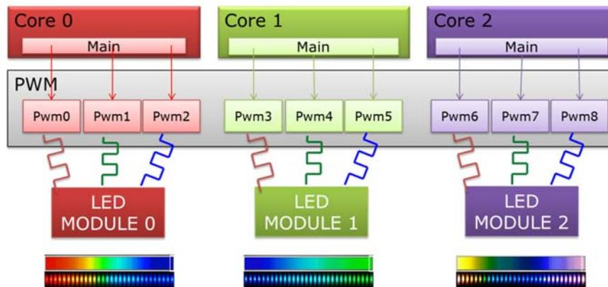
**Fig. 1.** Overview of dynamic LED system based on multi-core architecture
