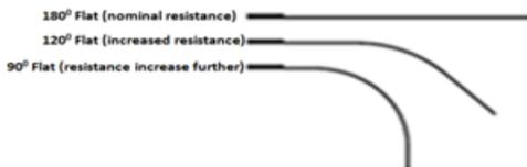
**Figure 3.** Bending Degree of Bending Sensor[2]
