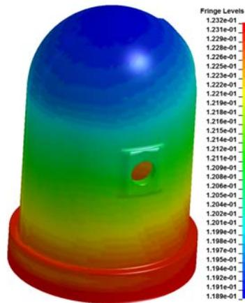
Figure 5: Displacements [m] in the containment structure under seismic load corresponding to a maximum design earthquake of magnitude 7.
