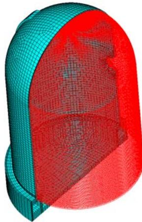
Figure 2: Computational model of the reinforced concrete structure of the NPP inner containment.
