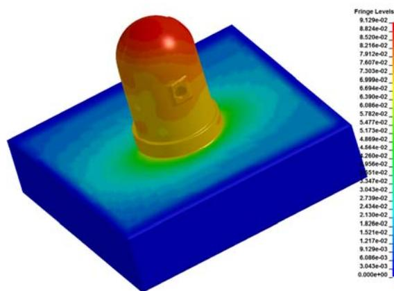
Figure 3: Velocities [m/s] in the containment structure and soil under seismic load corresponding to a maximum design earthquake of magnitude 7.
