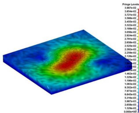
Figure 6: Accelerations [ $m / s^2$ ] in the lower soil section under seismic load corresponding to a maximum design earthquake of magnitude 7.
