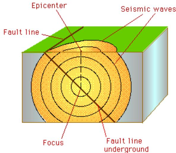
Figure 1: Schematic representation of an earthquake origin.
