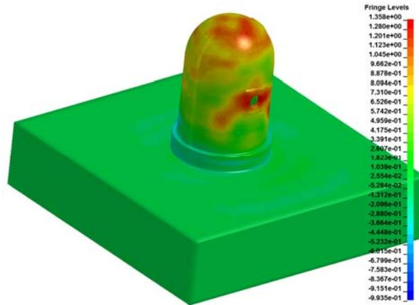
Figure 4: Accelerations [ $m / s^2$ ] in the containment structure and soil under seismic load corresponding to a maximum design earthquake of magnitude 7.
