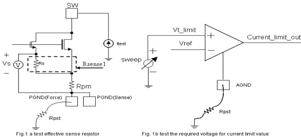
Fig.1 principle schematic of testing current limit value with voltage mode
