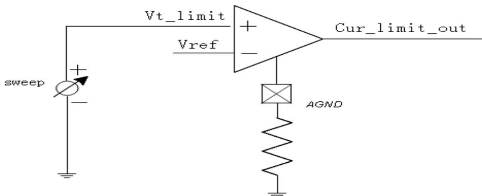
Fig.3 principle schematic for the required voltage of current limit value
