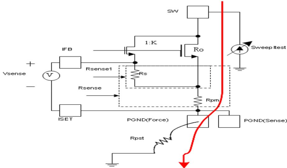
Fig.2 test schematic about sense resistor value
