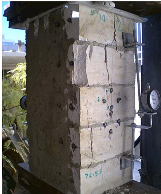
Figure 3: Typical compressive failure mode (hard stone).
