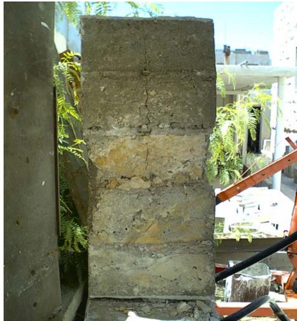
Figure 5: A typical longitudinal crack passing through the position where the wooden wedges were placed (broken stones were removed after failure)
