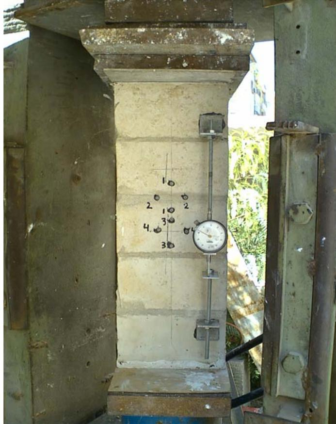
Figure 2: A five-course height prism with strain and displacement measurements
