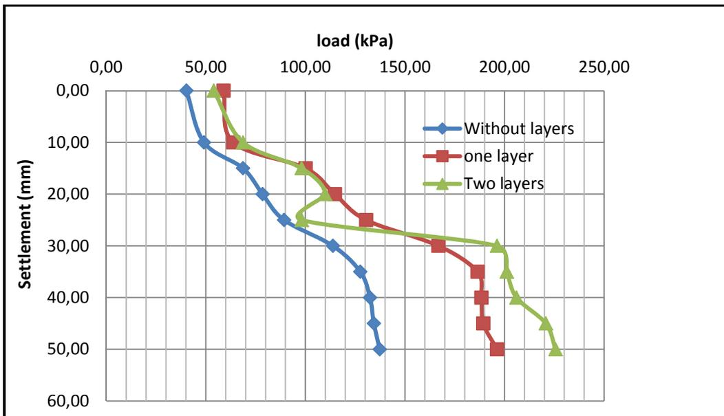
Fig.7: Load- Settlement of clay reinforced with geogrid SS2
