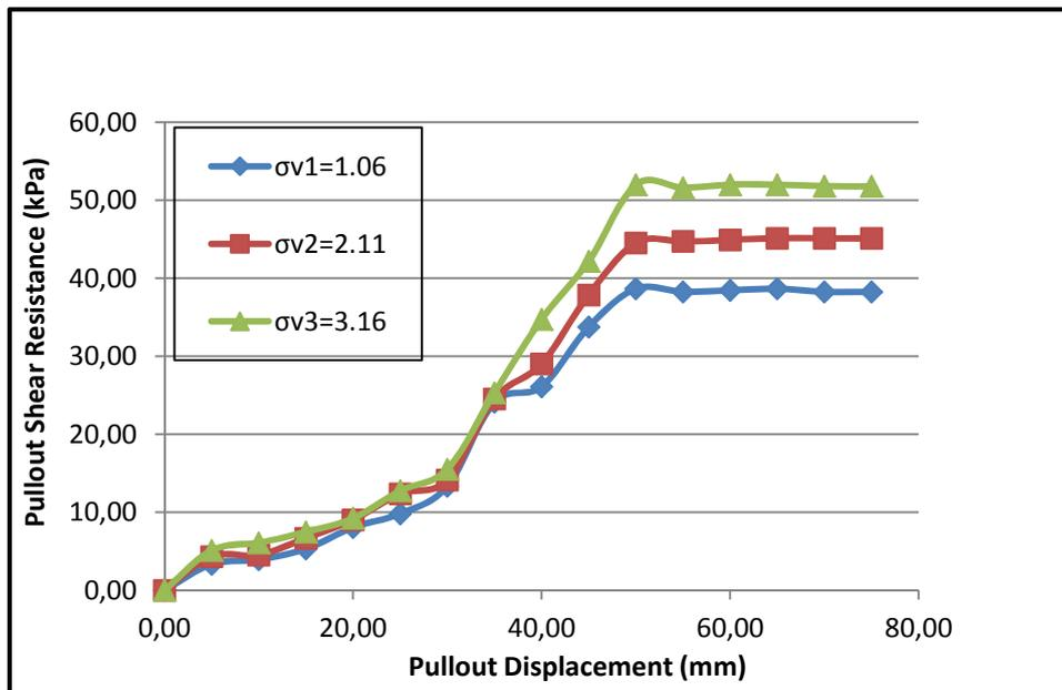
Fig.4: Pull-out test resistance of brown clay using SS2 Geogrid.
