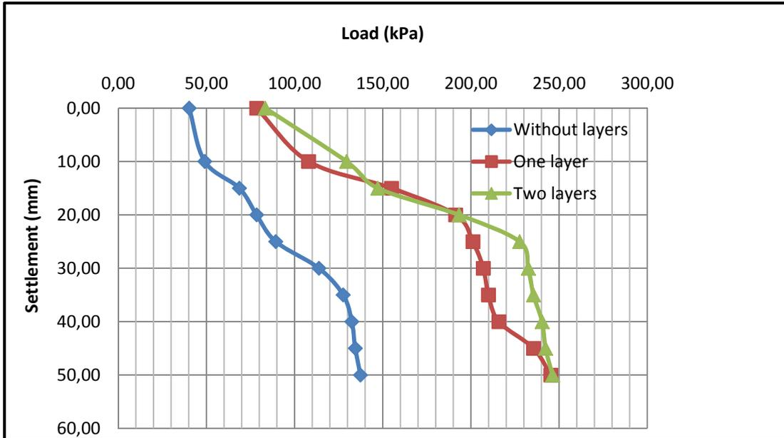
Fig.6: Load- Settlement of clay reinforced with geogrid SS40
