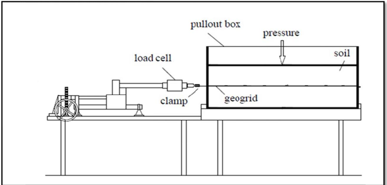
**Fig.2: A schematic Diagram of the pullout testing Apparatus.**
