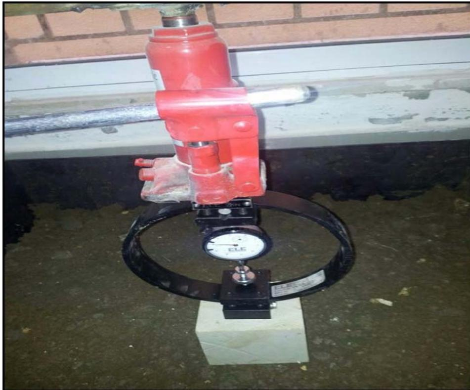
**Photo1: Load settlement test set up**
