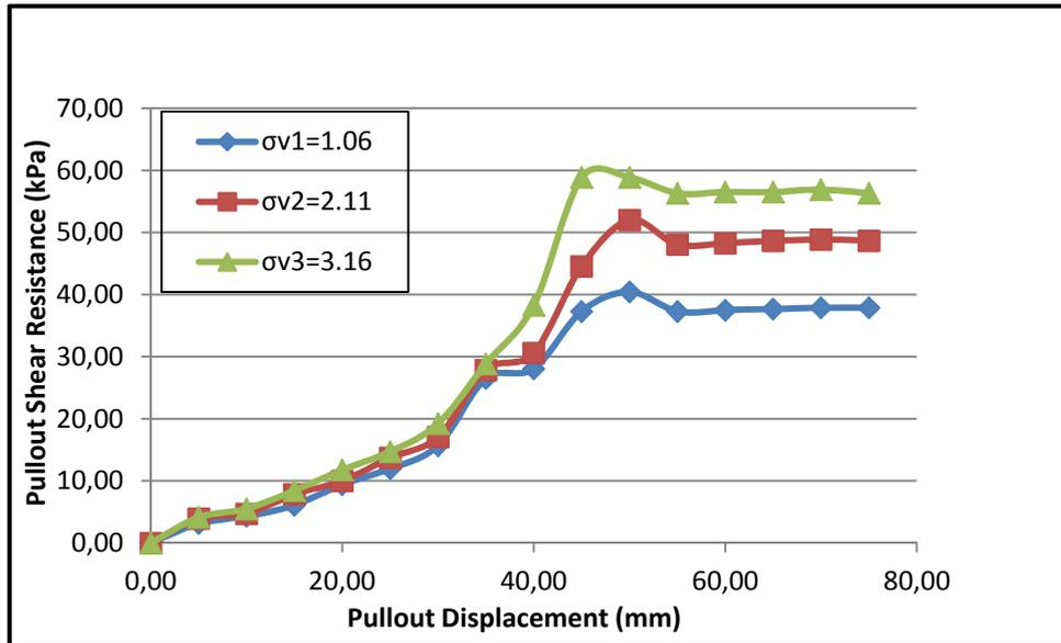
Fig.3: Pull-out test resistance of brown clay using SS40 Geogrid
