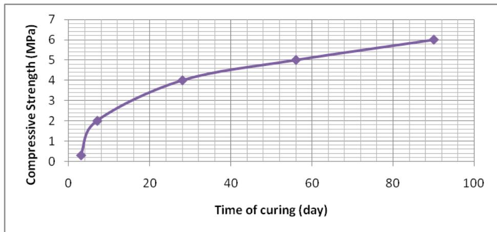
Figure 10: Compressive strength vs. time of curing for design mix No. 6
