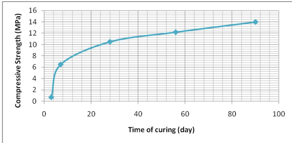
Figure 8: Compressive strength vs. time of curing for design mix No. 4
