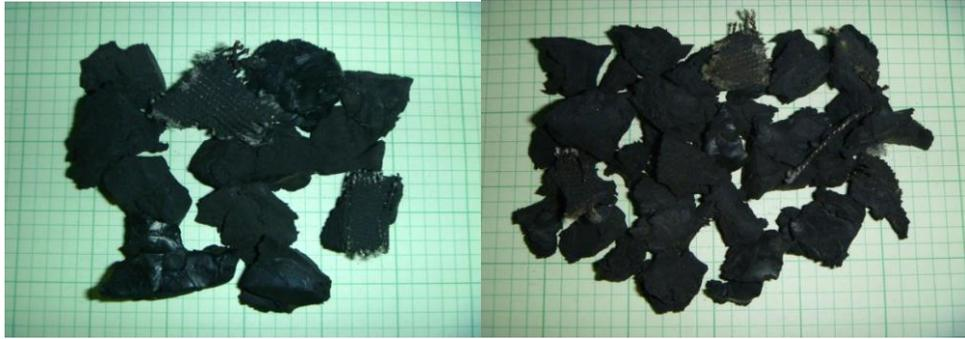
**Figure 1:** Shredded tires (25mm)      **Figure 2:** Shredded tires (19mm)
