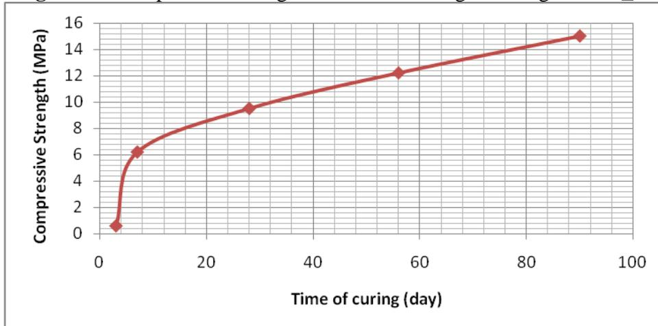
**Figure 6:** Compressive strength vs. time of curing for design mix No. 2
