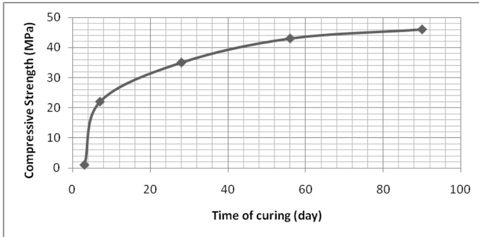
**Figure 5:** Compressive strength vs. time of curing for design mix No. 1
