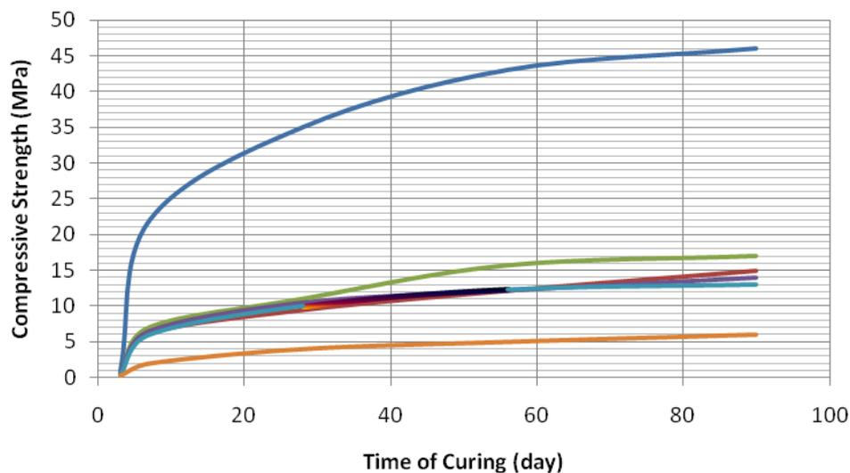
**Figure 4:** Compressive strength for all design mixes tests
