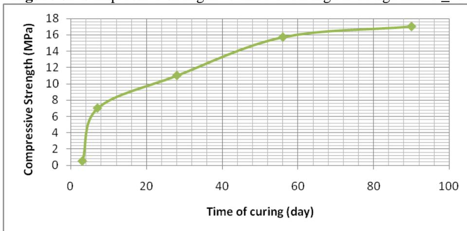
**Figure 7:** Compressive strength vs. time of curing for design mix No. 3
