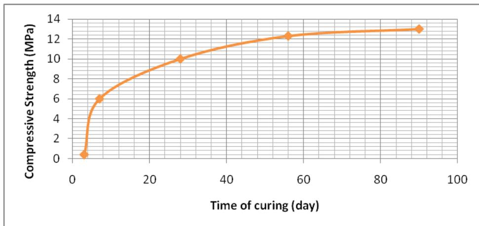
Figure 9: Compressive strength vs. time of curing for design mix No. 5
