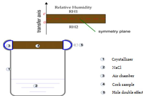
Figure 3: vaporimeter schematic
