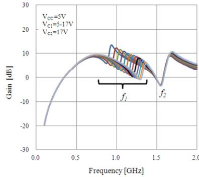
Fig. 17 Measured gains of the frequency-tunable dual-bandstop differential amplifier for a variable  $V_{C1}$  ( $C_{V1}$ ) and a fixed  $V_{C2}$  ( $C_{V2}$ )
