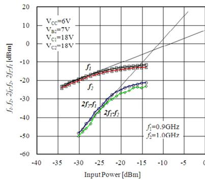
Fig. 13 Measured  $IIP_3$  performances of the frequency-tunable dual-bandpass differential amplifier
