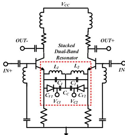
Fig. 14 Schematic diagram of the L-band SiGe HBT frequency-tunable dual-bandstop differential amplifier
