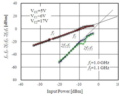
Fig. 19 Measured IIP<sub>3</sub> of the frequency-tunable dual-bandstop differential amplifier
