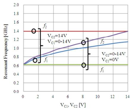
Fig. 7 Measured resonant frequencies of  $f_1$  and  $f_2$
