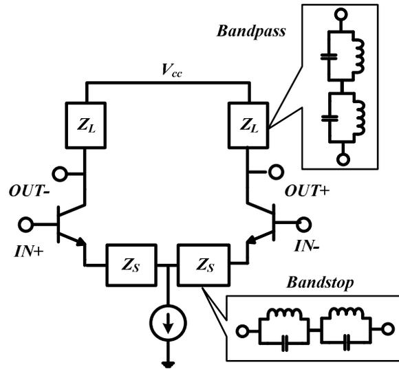
Fig. 1 Schematic diagram of the differential amplifier with the output circuit  $Z_L$  and the series feedback circuit  $Z_S$
