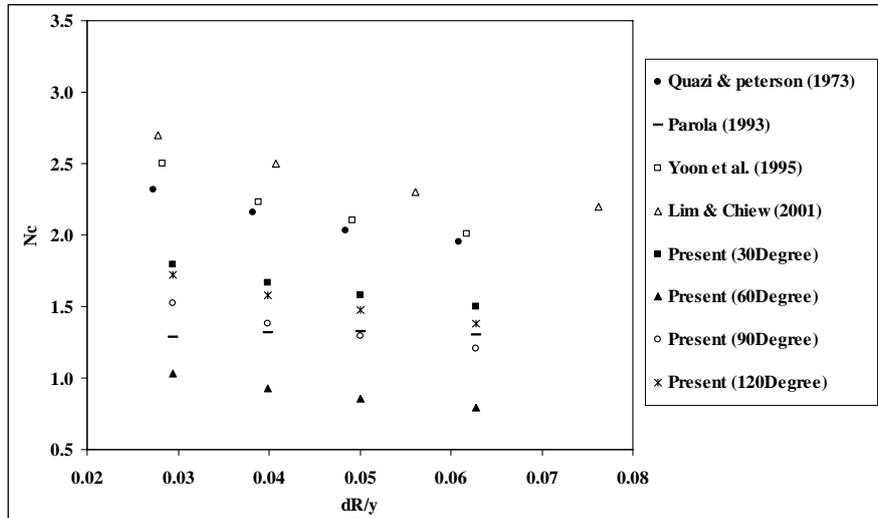
Figure 6. Comparison of riprap failure proposals in direct channels with present result
