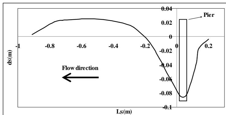
Figure 2. Longitudinal scour profile in position 60 degree
