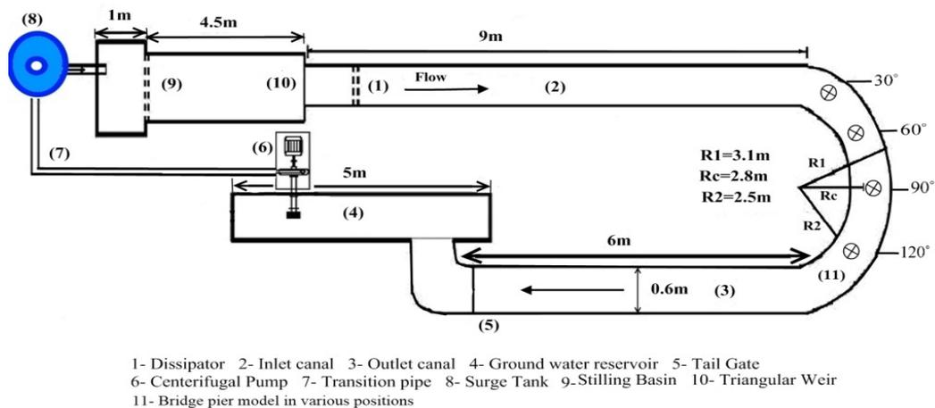
Fig. 1 Layout of Physical hydraulic model
