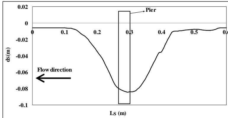
Figure 3. Transverse scour profile in position 60 degree
