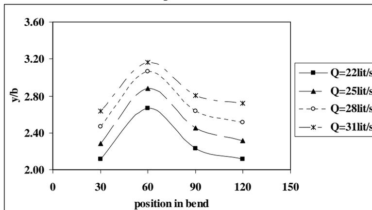
Figure 5. Relative flow depth versus cylindrical pier positions at the bend for various flow rates at the point of threshold conditions
