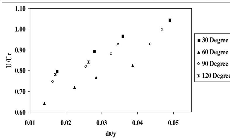
Figure 4. Critical velocity ratio against relative riprap diameter on different positions
