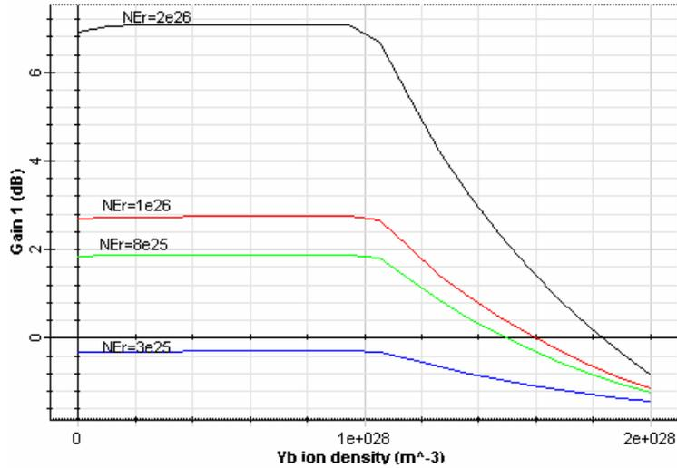
Figure (2) gain as a function of ytterbium concentration, back directional pumping with 200mW.
