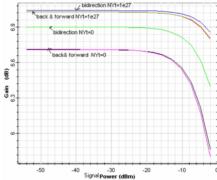
Figure (5) Gain as a function of signal power at different Yb-concentration and pump power configurations
