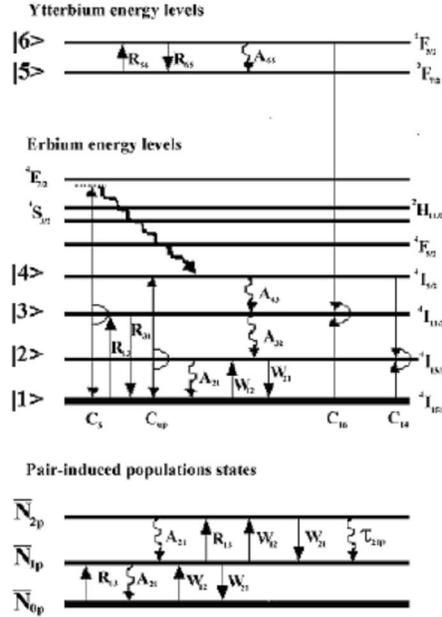
Figure (1) Coupled  $\text{Er}^{3+}/\text{Yb}^{3+}$  system, pumped in 980nm region
