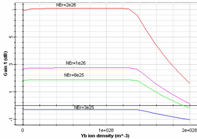
Figure (3) Gain as a function of ytterbium ion concentration, bidirectional pumping with 100mW in each direction
