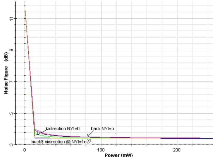
Figure (4-b) Noise figure as a function of pump power with backward and bidirectional pumping
