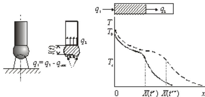
Fig. 2. Heating consumption in exchanging within the drop
