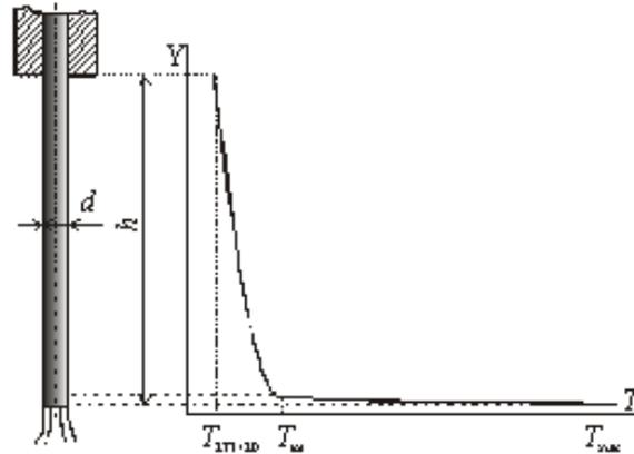
Fig. 1 Scheme of temperature distribution over electrode extension
