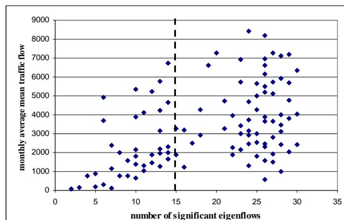
**Fig. 4. Relationship between number of significant eigenflows and monthly average daily traffic**
