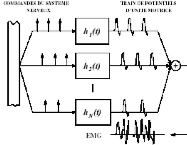
Figure 1: Schema of EMG model
