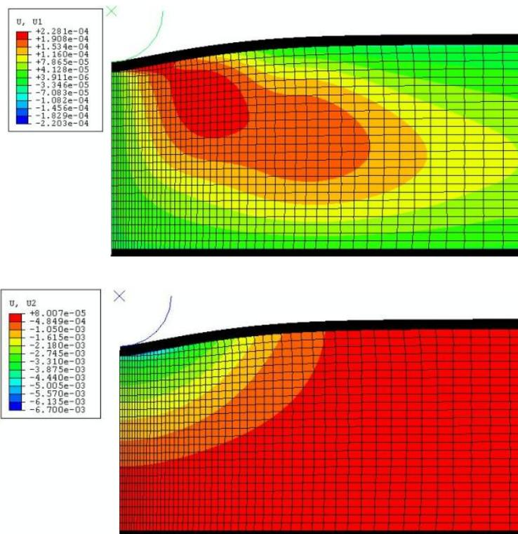
Fig. 5. Evolution of the displacement field deduced from the simulations at indentation of 7 mm.
