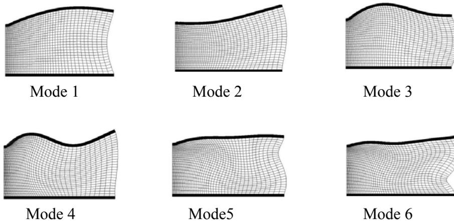
Fig.7. Examples of the shapes of the vibration modes of the composite sandwich panels.
