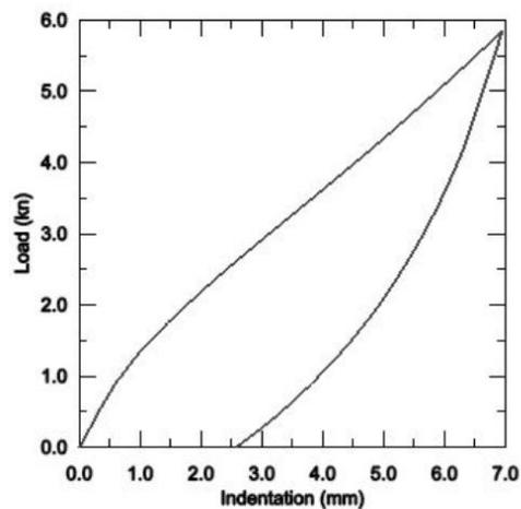
Fig. 3. Load-indentation curves deduced from the finite element modeling.
