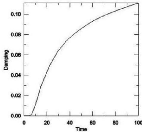
Fig. 8. Damping obtained for composite sandwich panel with PVC foam core.
