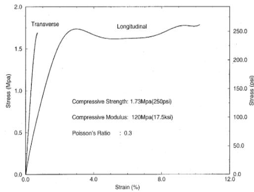
Fig. 2. stress-strain curves for Divinacell H100 Foam core under uniaxial compression.
