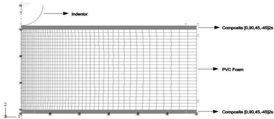
Fig. 1. Axisymmetrical finite element model of a sandwich panel indented by a spherical indenter.
