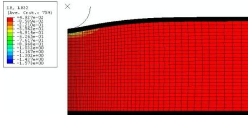
Fig. 6. Distribution of the vertical strain  $\epsilon_{22}$  corresponding to an indentation of 7 mm obtained in the finite element analysis.
