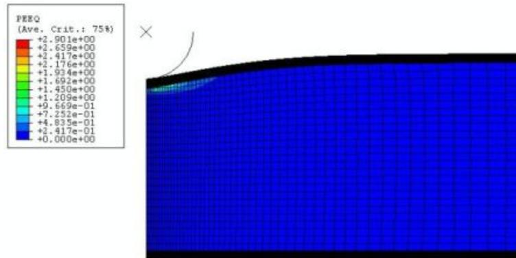
Fig. 4. Predicted contours of the volumetric compacting plastic strain in the foam core of a sandwich at indentation of 7 mm.
