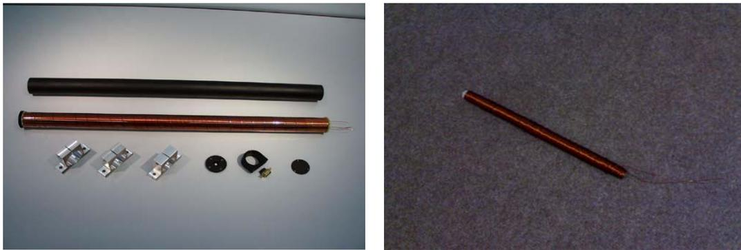
Figure 1: a separate magnetic torquer
