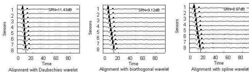
Figure 5: The obtained results by different wavelets (presence of delay and phase shift)
