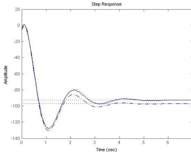
Figure 3. Step responses: original model (solid), reduced model using [3] (dash-dotted) and reduced model using the proposed framework within  $[1, 1000]$  frequency bound (dotted)
