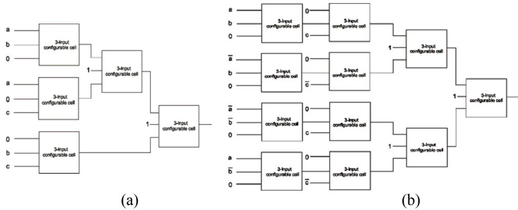
Fig. 15. A full adder block diagram based on three-input configurable cell. (a)Carry function diagram (b)sum function diagram.
