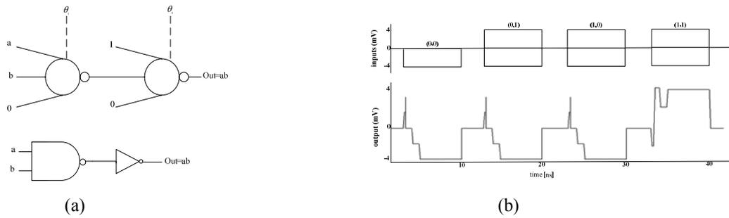
Fig. 7. (a) The AND gate and the gate schematic. (b) The simulation result for four sets of inputs.
