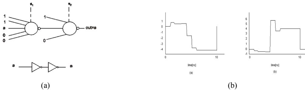
Fig.11. (a) a buffer based on two majority gates in series. (b) The simulation results for the proposed buffer.
