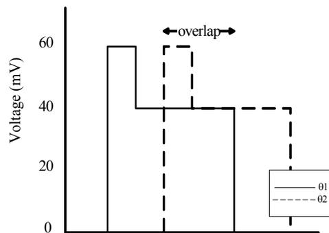
**Fig. 5.** the two-phase two-step clock pulses used to excite majorities.
