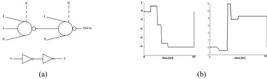
**Fig. 6.** (a) Buffer based on two majority gates in series, and the gate schematic.(b) the simulation results for proposed buffer.
