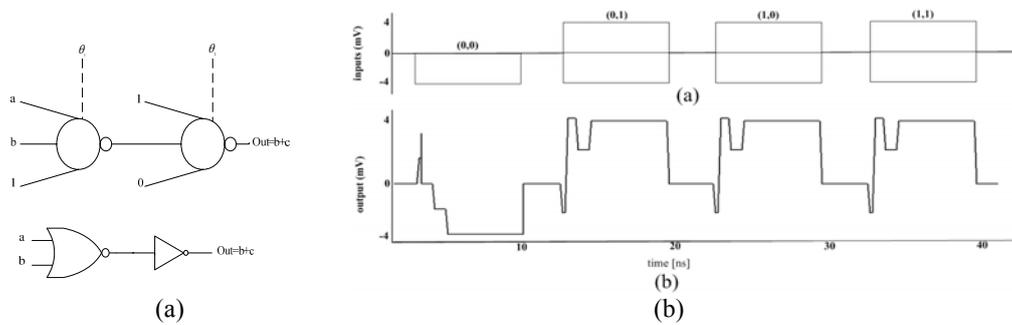
Fig. 8. (a) The OR gate and the gate schematic. (b) The simulation result for four sets of inputs.
