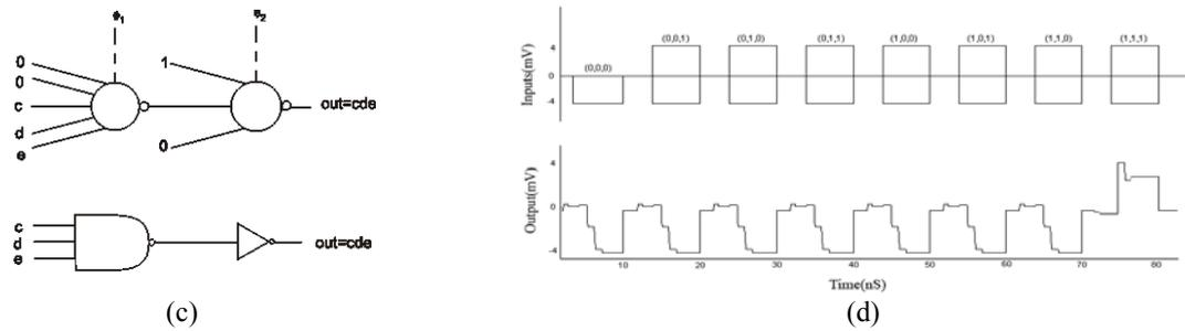
**Fig.12.**(a) The two-input AND gate and the gate schematic. (b) two-input AND gate simulation for four different sets of inputs. (c) The three-input AND gate and the gate schematic. (d). AND gate simulation for eight sets of inputs.
