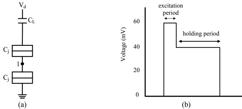
**Fig.1.**(a) An irreversible single electron box (SEB) with a double tunnel junction [6].(b) a two-step pulse that shows excitation and holding period (selected from [4]).
