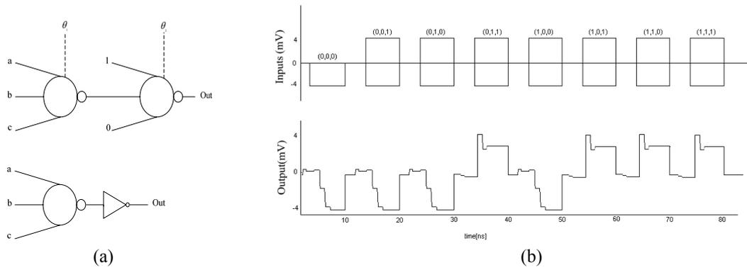
**Fig. 4.** (a) three-input majority gate with two complementary majority gates in series that the second majority acts as NOT gate. Two-step clock pulses controls signal flow (b). Simulation results for three-input majority gate.
