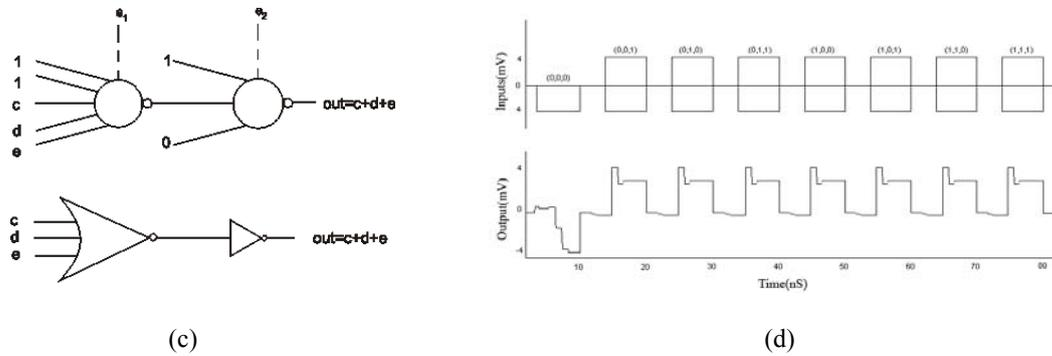
**Fig.13.**(a) The two-input OR gate and the gate schematic.(b) two-input OR gate simulation for four sets of inputs. (c). The three-input OR gate and the gate schematic.(d) three-input OR gate simulation for eight sets of inputs.
