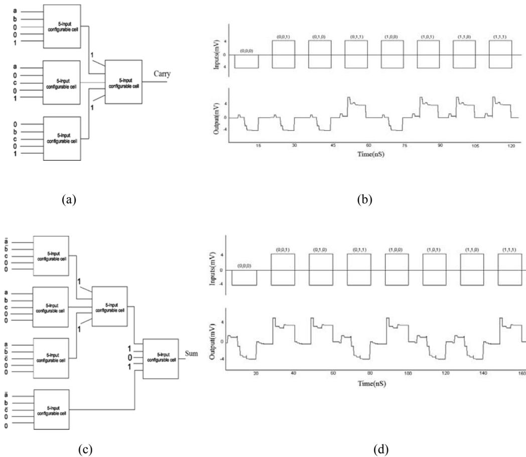
**Fig. 14.** A full adder block diagram based on five-input configurable cell. (a) Carry function diagram (b) Carry function simulation results (c) Sum function diagram (d) Sum function simulation results.
