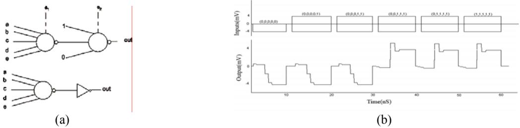
**Fig. 10.** (a) A five-input majority gate and the gate schematic. (b) The simulation result for proposed majority gate with five different inputs.
