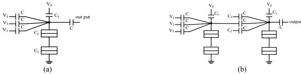
**Fig.2.**(a) a complementary majority gate based on irreversible single electron box [6].(b) a novel three-input cell for producing different logic by applying appropriate voltage (logic levels) to the inputs.
