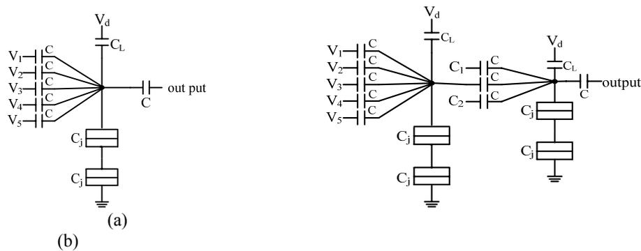
Fig.9.(a). A five- input complementary majority gate based on irreversible single electron box. (b) A new five-input configurable cell.
