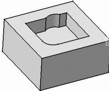
Fig. 7: Irregular Pocket with uniform depth 50 mm in a block
