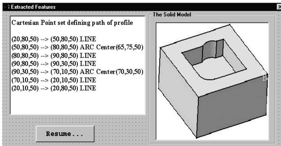
Fig. 8: Output of Irregular pocket after analyzing the STEP file
