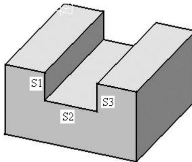
Fig. 3: Rectangular Slot 100 X 20 X 10 mm in a block
