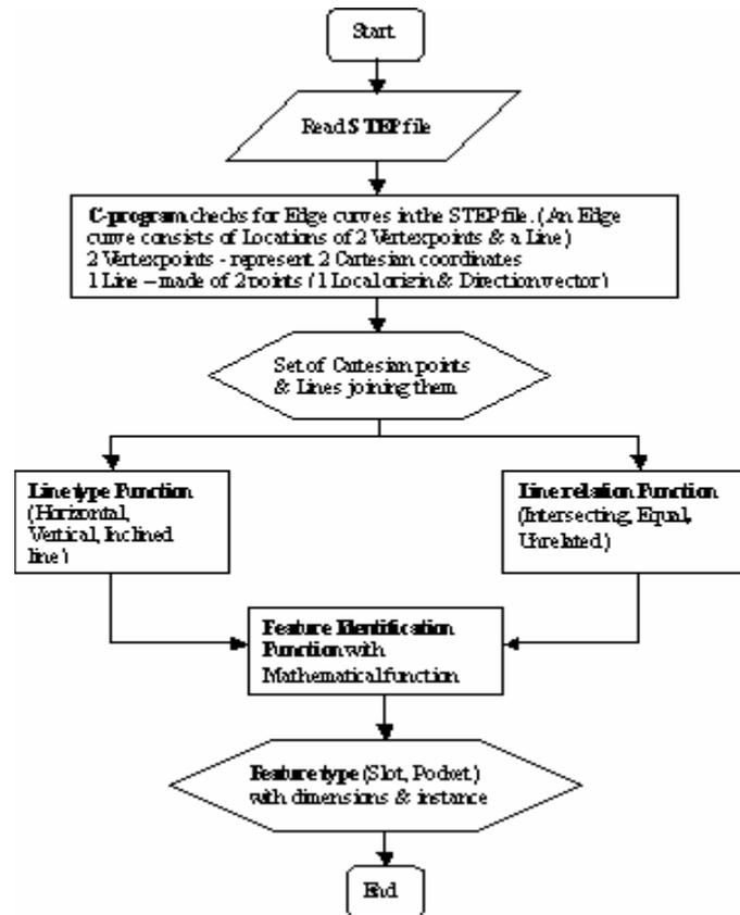
Fig. 5: Flowchart depicting the Logic used in programming
