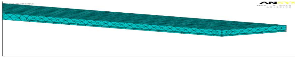
Fig.5. Mesh of a delaminated beam by ANSYS.
