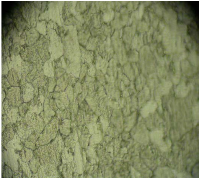
Fig( 3 ) microstructure of raw plate before galvanization
