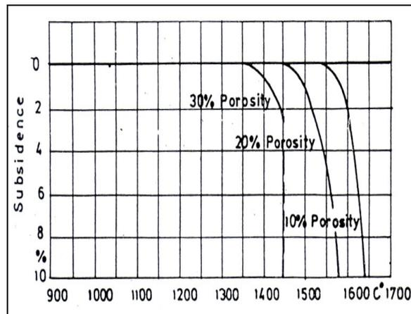
Fig.2 Influence of Porosity on the Refractoriness under Load of Fire-Clay Bricks
