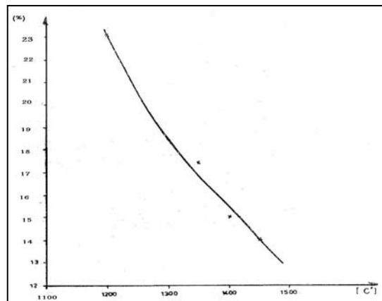
Fig.10 Relationship between the porosity and the firing temperature.
