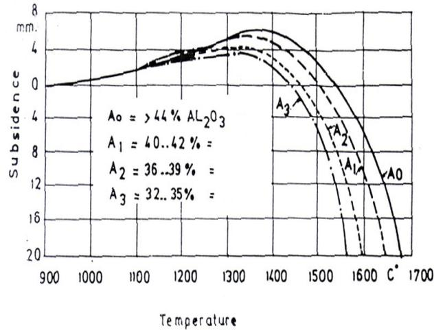
Fig.1 Influence of  $Al_2O_3$  Content on the Refractoriness under Load of Fire-Clay Bricks.
