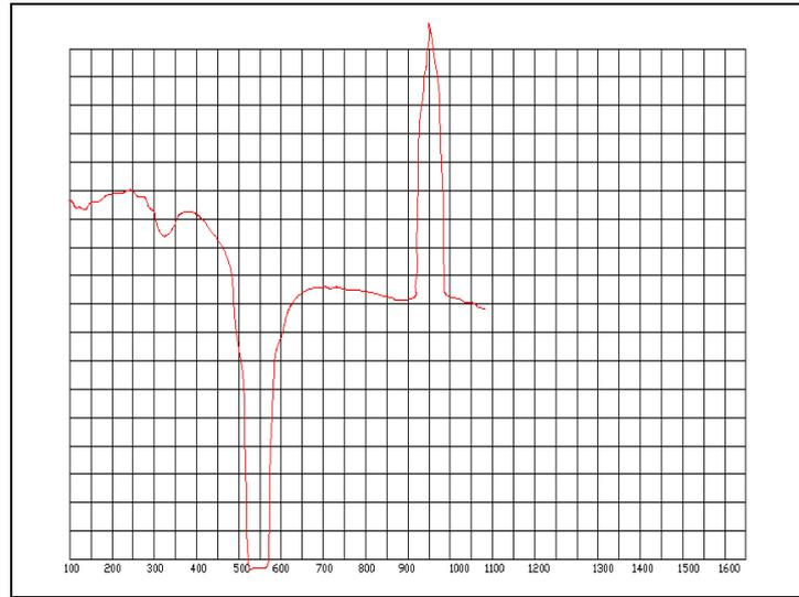
Fig, 9 Differential Thermal Analysis of our Clay.
