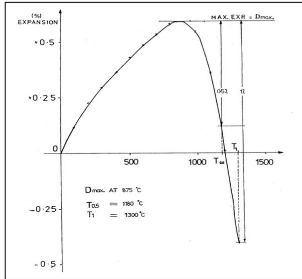
Fig. 11 Refractoriness Under Load of The Alumina Free Sample.
