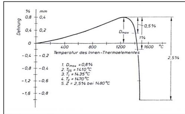
Fig.3 The Rate of sagging of the Brick with Temperature Size.
