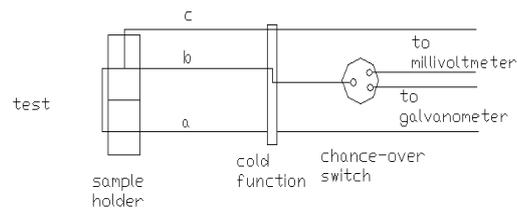
Fig.4 differential thermal analysis apparatus. The Specimen holder and the chromo-couple arrangement.
