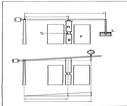
Fig. 8 Measuring Refractoriness Under Load.
