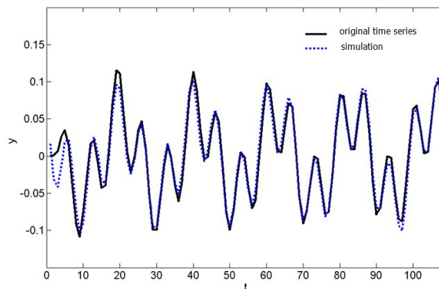
Fig. 2 Comparison of the dynamics of the model and the system (solid line — dynamics of the original system, dotted — simulated by the model signal)
