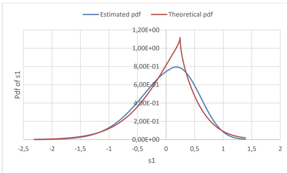
**Figure 1.** Estimated and theoretical marginal pdf of  $s_1$  in the bivariate Weibull model with parameters  $\lambda_1 = \lambda_2 = 1, \gamma_1 = \gamma_2 = 1.5$  and  $\alpha = 0.8$ . ( $n = 100$ )
