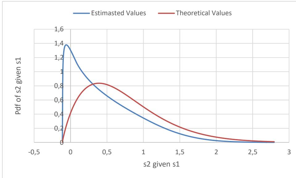
**Figure 2.** Estimated and theoretical pdf of  $s_2|s_1 = s_1^*$  in the bivariate Weibull model with parameters  $\lambda_1 = \lambda_2 = 1, \gamma_1 = \gamma_2 = 1.5$  and  $\alpha = 0.8$ . ( $n = 100, s_1^* = -1.5$ )
