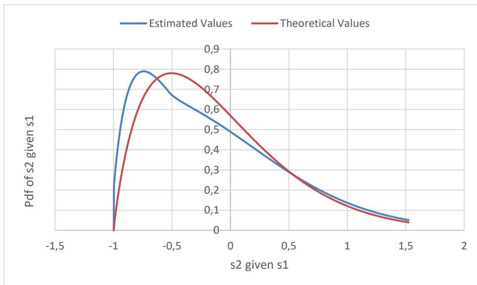
**Figure 3.** Estimated and theoretical pdf of  $s_2|s_1 = s_1^*$  in the bivariate Weibull model with parameters  $\lambda_1 = \lambda_2 = 1, \gamma_1 = \gamma_2 = 1.5$  and  $\alpha = 0.8$ . ( $n = 100, s_1^* = -0.1875$ )
