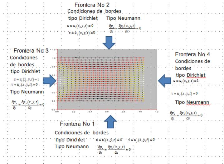
Figure 1 Laminar flow between parallel planes with edge conditions
