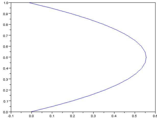
Figure 3 Laminar flow velocity profile between parallel planes
