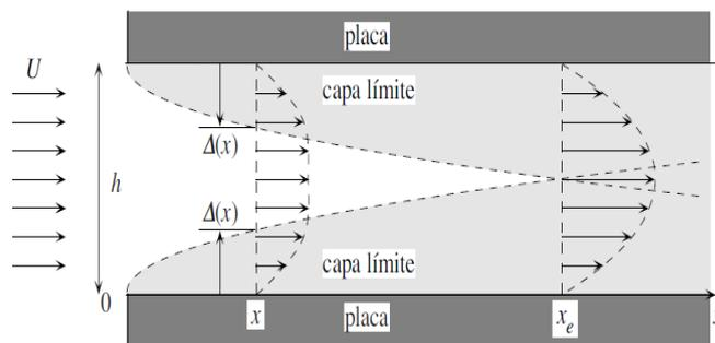
Figure 2 Embouchure effect for the flow between semi-infinite flat plates: evolution of the velocity profile with the distance from the entrance
