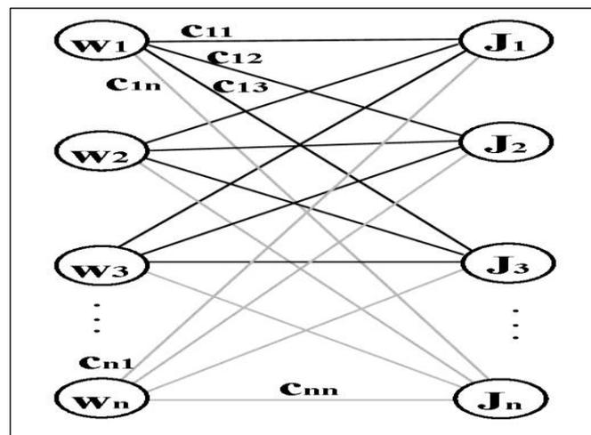
**Figure (1):** Network representation of the assignment problem
