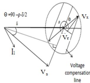
Figure 2. Vector diagram of IPFC
