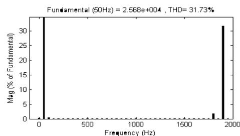
Figure. 6. THD of converter output voltage
