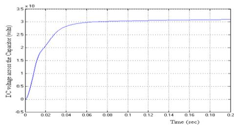
Figure 8. DC link voltage with PI Controller
