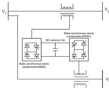
Figure 1. Schematic diagram of IPFC
