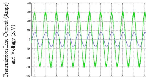
Figure. 7. Transmission line current and voltage
