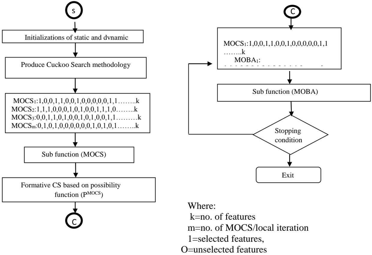
Figure 1. Hybrid Algorithm Flow chart
