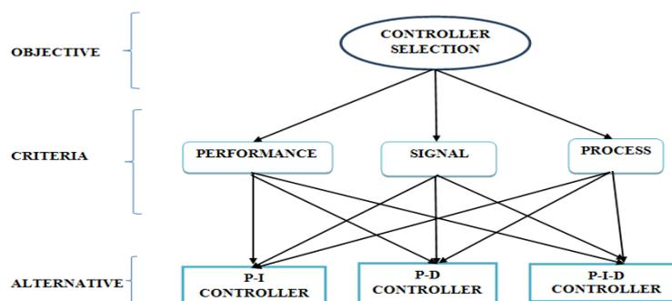
The Figure-1 clearly shows the hierarchical structure for cascade control system using AHP. The highest level describes the goal here we are thriving for selection of optimal controller. The succeeding level in AHP hierarchy illustrates criteria's taken into consideration namely performance, signal, and process. The lowest level of the hierarchy reveals the alternative namely P-I-D, PI, PD controller.
