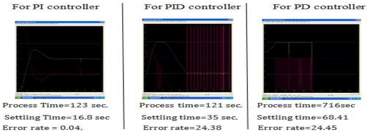
Figure 2 illustrates that the error rate of PI controller is much lesser than that of PID and PD with less settling time that urges to be chosen as an optimal controller in a manufacturing organization.
