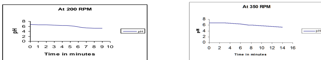
FIGURE4 Response for pH for step change in speed of Magnitude 150 rpm
