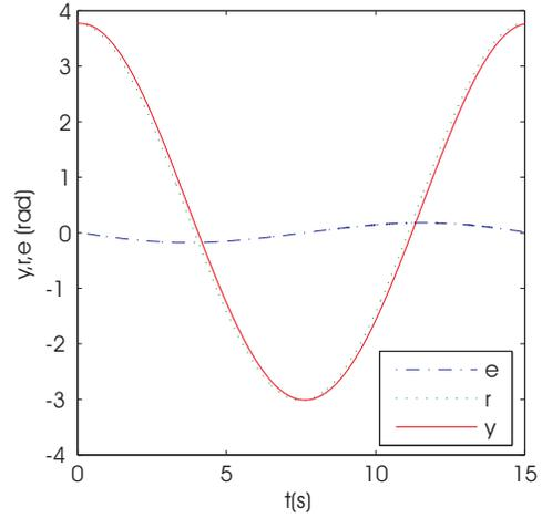
Figure 4: Reference (r), output (y) and error (e) of the actuator at  $J = 0.025 \text{ kg m}^2$
