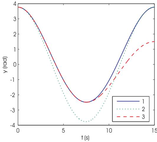
Figure 3: Symmetric semiprogram motion (1), free undamped motion (2), free damped motion (3)
