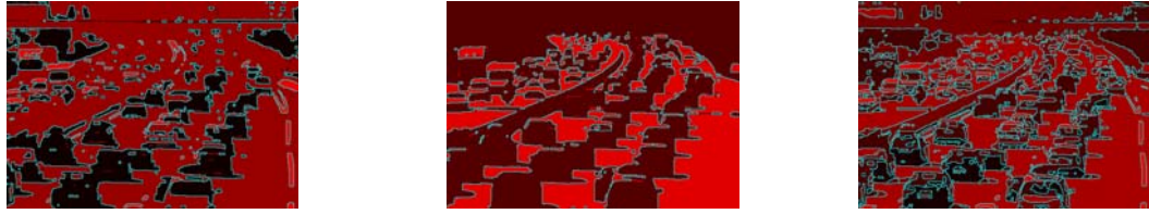
Figure 5: Representation of watersheds applied to the three gradients. From left to right: the watershed associated to the gradient of the hue channel, the watershed associated to the gradient of the saturation channel and the watershed of the gradient of the intensity channel.
