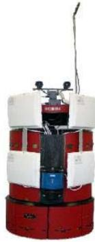
Figure 3: A mobile robot equipped with RFID antennas
