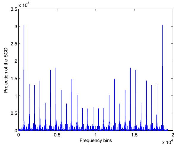
Figure 3: The cyclic spectrum of the GRF signal
