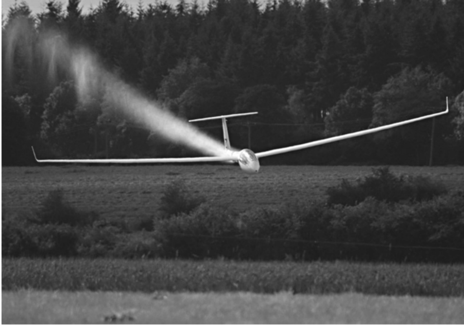
Fig. 2 Water ballast dropping of sailplane (from [14])
