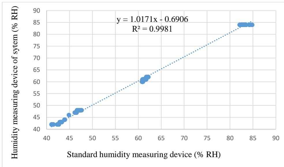
**Figure 3.1** Relation between standard humidity measuring device and humidity measuring device that has been designed
