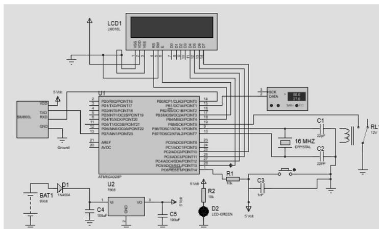
**Figure 2.1** The complete design of humidity monitoring system for oyster mushroom cultivation room by web based AVR ATmega328P-PU
