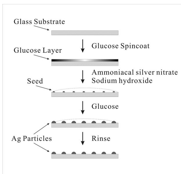
Figure 1. Schematic drawing of reduction position controlled (RPC) method.
