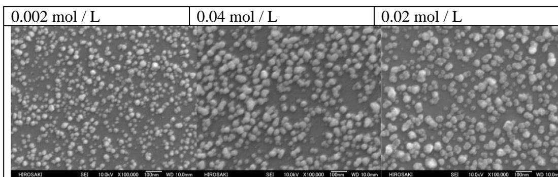
Figure 3. SEM images of silver fine particle films produced by the glucose concentration during spin coating
