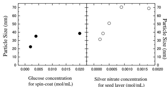
Figure 4. Silver particle size as a function of glucose concentration for spin-coat and silver nitrate concentration for seed layer formation.
